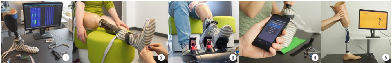
Figure 1. With proCover, we present a novel concept for prosthetic-sensing wearables (1) based on smart textiles that allows amputees to “feel” again (2). In our studies, participants had less difficulties while performing the tasks with proCover (3). A mobile app enables user-driven creation and mapping of sensing regions (4). Finally, the sensor can also be used for tracking bodily positions (5).
