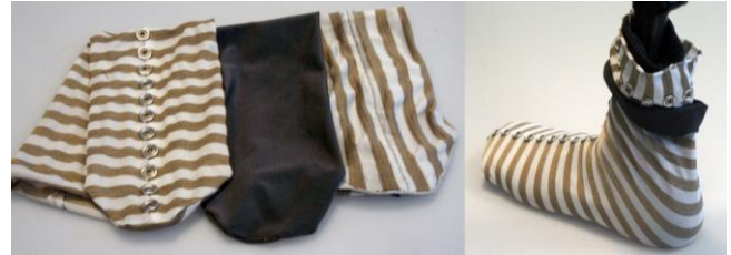
Figure 3. Prototype of the textile-based sensing sock
