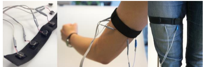
Figure 4. Array of vibration motors used for haptic feedback. The motors can be attached to different bands, which can be worn on different body parts like the upper arm or thigh.
